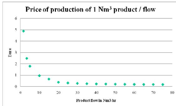
**Figure 11: Product price per Nm<sup>3</sup> (in Euros) of upgraded gas for various production flows.**
