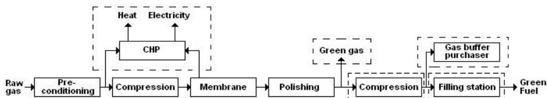
**Figure 9: Schematically impression small scale membrane installation**
